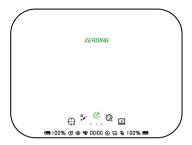
Take a shot, make the cross center of the reticle at point of impact. Short press **MENU/REC** button to switch zeroing options.
